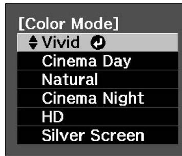
Press and select the color mode from the menu. Setting is also possible using the configuration menu.
