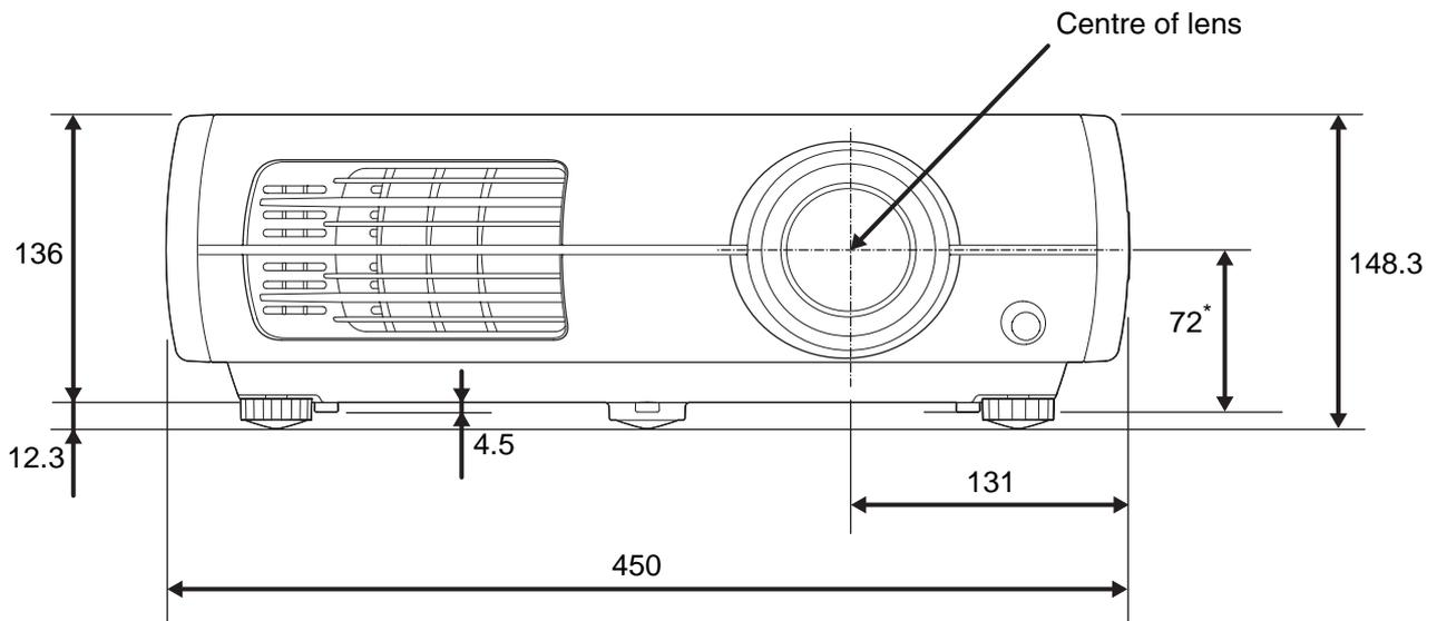
\* Distance from centre of lens to suspension bracket fixing point
