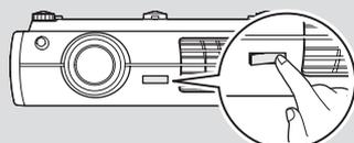
When one end of the plate is pressed, the opposite end lifts up, so you can pull it out slightly, turn it around and then push it back in.
