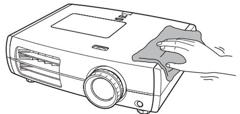
**Attention** Do not use volatile substances such as wax, alcohol or thinner to clean the projector case. These can cause the case to warp and make the coating finish peel off.
