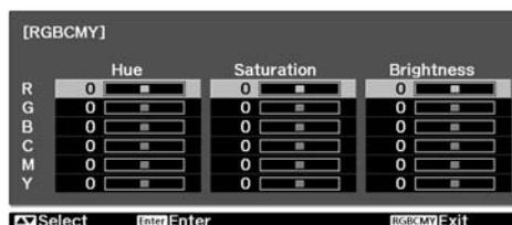
The hue, saturation, and brightness for each of the R (red), G (green), B (blue), C (cyan), M (magenta) and Y (yellow) color components can be adjusted. Adjustment is not possible when "Color Mode" is set to "x.v. Color".
