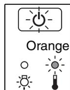
You can continue using the projector, but if the temperature rises again, it will switch off automatically.
