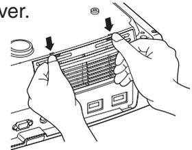
Press the knobs to release the catches, and then pull the cover upward.
