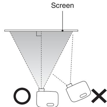
If the projector is placed at an angle to the screen, then the projected image will be distorted.
