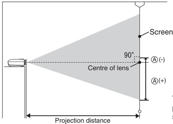
This is the height from the centre of the lens to the bottom of the projection images. It can be changed by the vertical lens shift setting.
