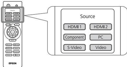
Press the button that has the name of the port on it that the desired signal source is connected to.
